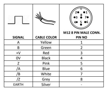
In the right table the cable colors of sensors output signals are given. If the control circuit is suitable in the Line Driver sensors of the not output signals (/A, /B, /Z) have to be added to the system. If it is not suitable /A, /B, /Z signal cables must be fixed as insulated separately. Don't forget that these edges have electricity too.
