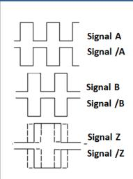
In the right table the cable colors of sensors output signals are given. If the control circuit is suitable in the Line Driver sensors of the not output signals (/A, /B, /Z) have to be added to the system. If it is not suitable /A, /B, /Z signal cables must be fixed as insulated separately. Don't forget that these edges have electricity too.
