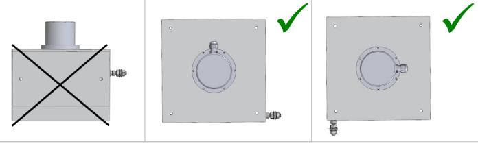
3. If there is a trickle of water (like a rain), the wire outlet must not be a drip of water upstream. If needed please use guide rollers.
